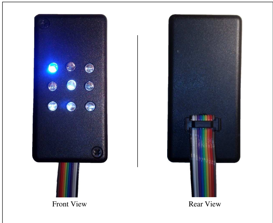
Figure 5-3: Fully Enclosed 3x3 LED-Grid Unit
