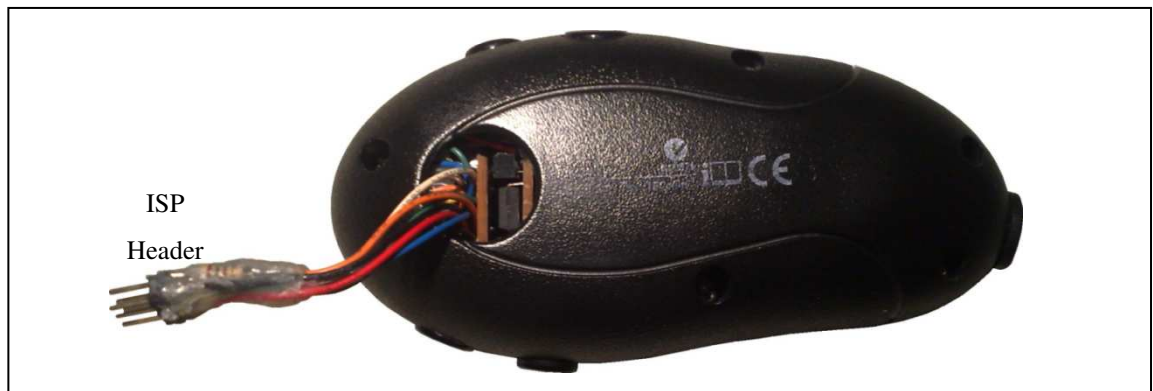
Figure 4-3: Assembled Transmitter-Unit with Externally Accessible ISP Header
